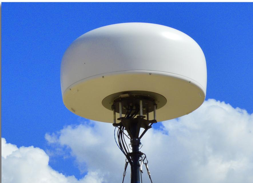
Each antenna is factory calibrated by Espy to support both AoA DF and TNG. Additional site calibration may be required for optimal TNG operations.
