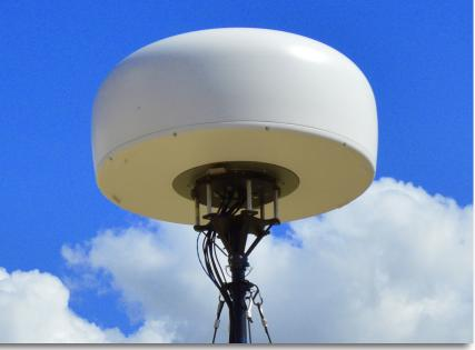
Each antenna is factory calibrated by Espy to support both AoA DF and TNG. Additional site calibration may required for optimal TNG operations.
