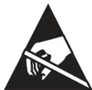
This device contains electrostatic discharge sensitive devices and is sensitive to electrostatic discharge (ESD). Observe all precautions for handling electrostatic sensitive devices.
